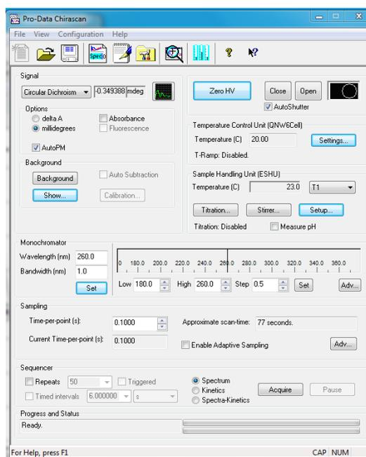
17. Loading the 1-mm-pathlength cuvette with 200 $\mu$ L buffer. Drag the file **5\_Buffer CD with Abs\_FarUV.dsx** to Chirascan window and change file name in spectrum block. Insert the cuvette at cell 1 position and click **Acquire** to start the experiment.
