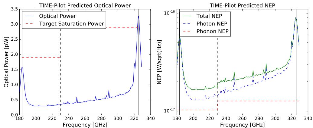
Figure 6. *Left:* The target detector saturation power and expected optical load for a single  $R \sim 100$  channel centered on the specified frequency assuming 1 mm PWV at the JCMT. *Right:* The expected total per-detector NEP. Phonon noise is sub-dominant to photon noise.
