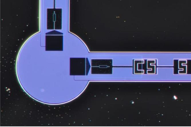
Fig. 1 The IDP SIS mixer with a planar OMT on the membrane. The transparent part is free standing membrane without covered metal. Two rectangular probes, turning circuit, SIS junctions, and RFCs are suspended on the membrane.
