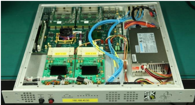
Fig. 2. ROACH with two 5-Gsps ADCs connected.
