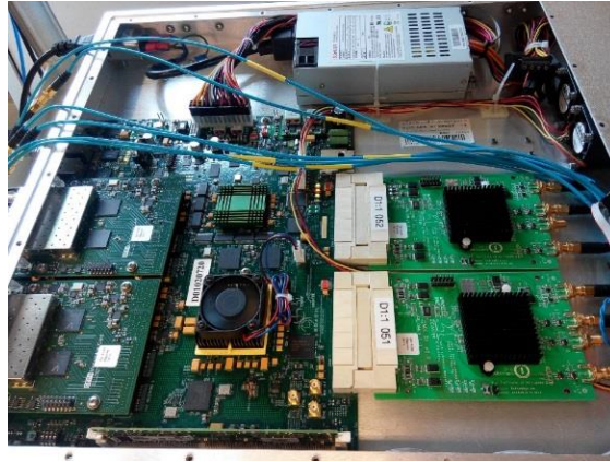
Figure 4. Digital hybrid implemented using the ROACH2 DSP module on the left and two 5 Gbps ADC boards on the right.
