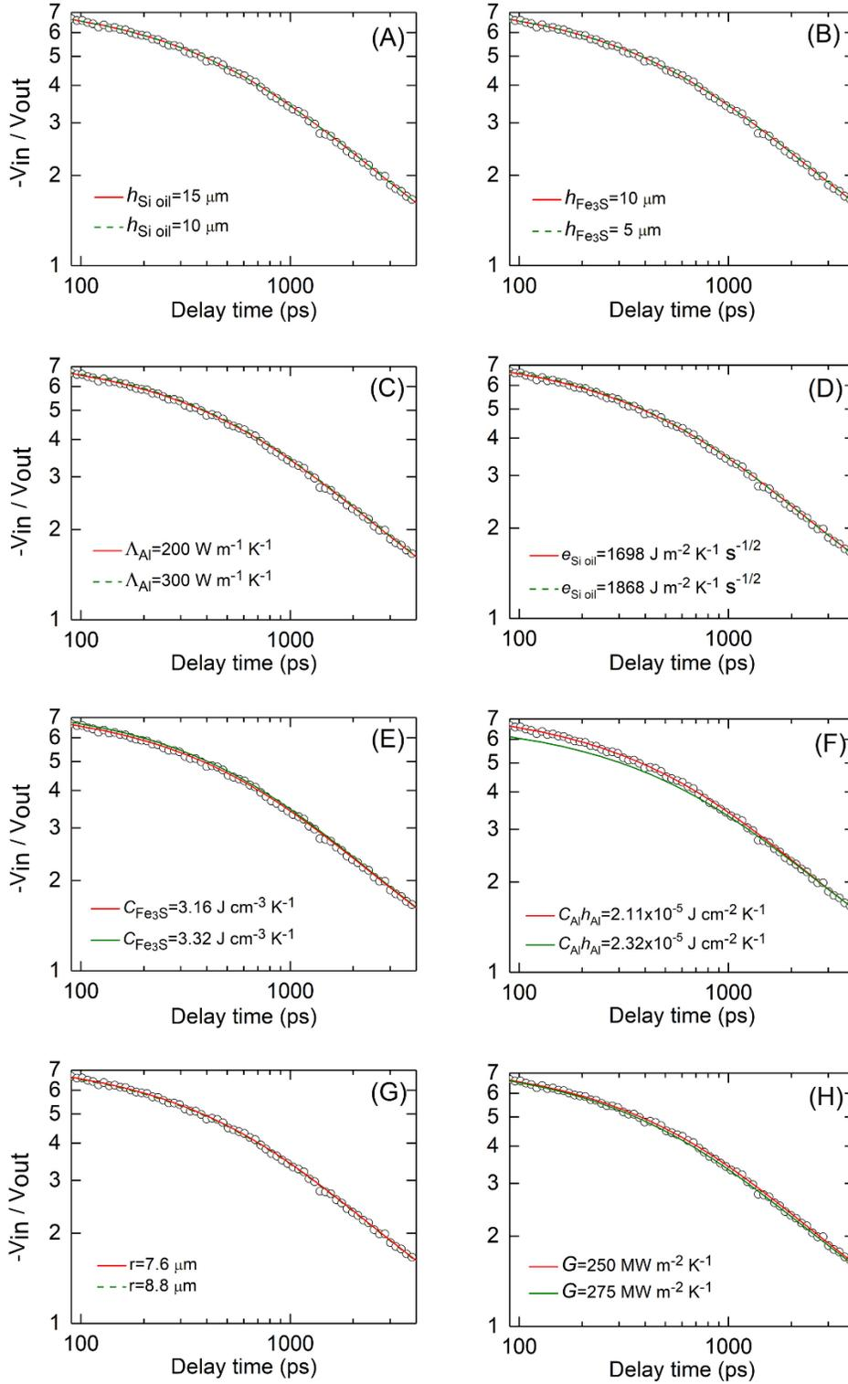
**Fig. S2.** Sensitivity tests of the thermal model to input parameters for Fe<sub>3</sub>S at 40.5 GPa. Thermal conductivity of Fe<sub>3</sub>S,  $\Lambda_{\text{Fe}_3\text{S}}$ , is fixed at  $25 \text{ W m}^{-1} \text{ K}^{-1}$ , as shown in Fig. S1. (A) and (B) Changes in the thicknesses of silicone oil ( $h_{\text{Si oil}}$ ) and Fe<sub>3</sub>S ( $h_{\text{Fe}_3\text{S}}$ ) by 33% and 50%, respectively, have
