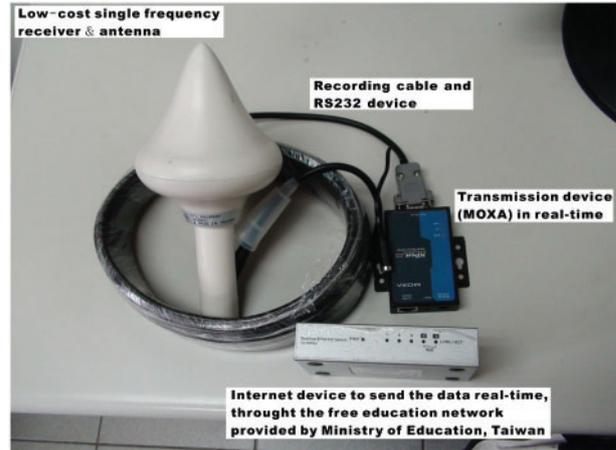
**3 Entire unit of low-cost single-frequency receiver and transmission devices**
