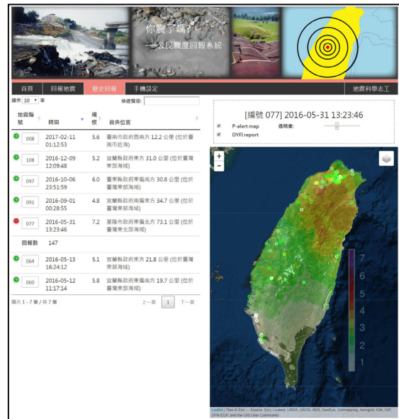
Fig. 6. An example of crowdsourced intensity for the 2016/05/31 Mw 6.4 event at DYFI@Taiwan. The shake map in colors is derived from P-Alert observations 2 .
