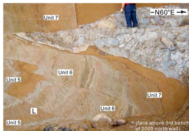
Figure 13. Detailed view of the NE end of the third bench of the 2005 north wall after the surface had been prepared for a plastic peel. The lowest of the two obvious faults is the lower main fault, identified as "L" in the text. It placed Unit 6 in lateral contact with Unit 5. The fault above, between two blocks of Unit 6, is termed medium-sized fault in the text.
