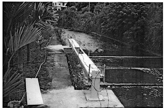
Fig. 3. Two different types of the surface installation of the base of the creepmeter. Upper figure: installation type I, concrete bases are planted vertically on the surface by digging a 0.5-m deep hole. Lower figure: installation type II, concrete bases are horizontally fixed on the water channel's wall.
